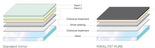
A paint providing unique protection against corrosion, abrasion and scratches.
